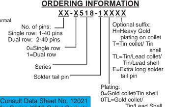
for Series X518 Collet Sockets with wire wrap pins.
